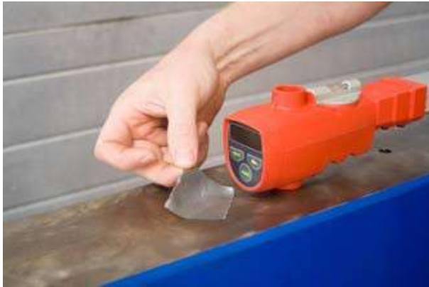
1. Mount tape on the surface.
