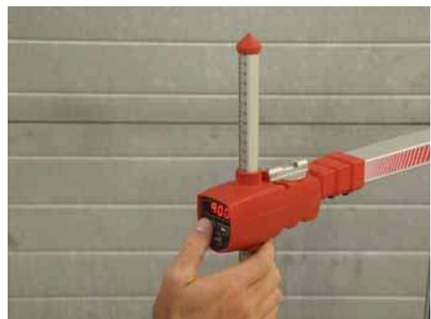
4. Snap in the tip/cup to height measuring rod.
