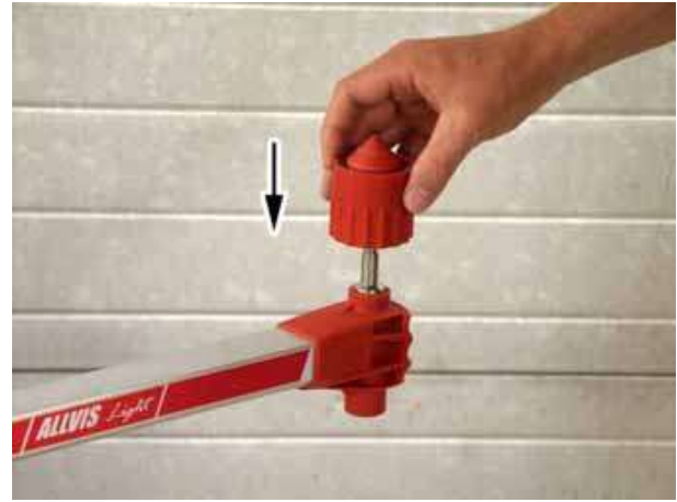
2. Snap on the magnet to the datum rod.
