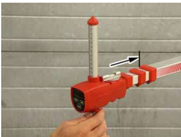
5. Compress the measuring arm.
